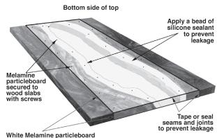
(pressed firmly onto bead of silicone sealant to remove trapped air)
